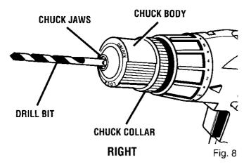
To tighten the chuck jaws on drill bit; grasp and hold the collar of the chuck with one hand, while rotating the chuck body with your other hand.
